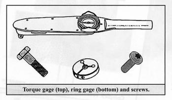
freely enter into a GO ring gage, very little torque is required to make them go through the gage.
